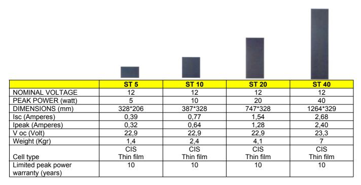
Power specifications are at standard test conditions (STC): irradiance level 1000w/m2, spectrum AM 1.5 and cell temperature 25oC
